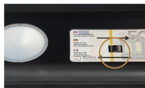
The magnetic sensor checks the magnetic characteristics of the security thread.
